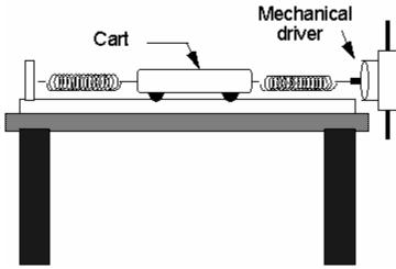
The mechanical driver is somewhat like a loudspeaker with one end of a metal rod attached to the center, and the other end of the rod is attached to one of the springs. The driver is connected to the signal generator that causes the rod to oscillate back and forth with adjustable frequencies that can be read off the display on the signal generator.
