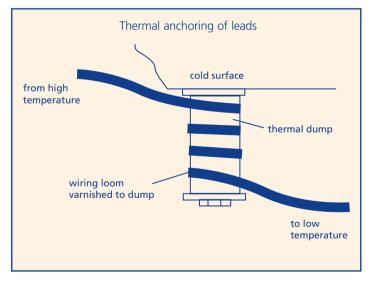
The same techniques can be applied to systems working at millikelvin temperatures. A heat load of 0.1  $\mu$ W is enough to produce noticeable warming at these temperatures.
