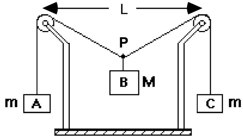
The system consists of a central object, B, suspended halfway between two pulleys by strings. The picture above is similar to the situation with which you will work. The objects A and C, which have the same mass ( $m$ ), allow you to determine the force exerted on the central object by the string. You do need to make some assumptions about what you can neglect. For this investigation, you will also need a meter stick and weights to vary the mass of B.
