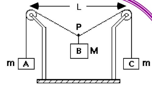
1. **Draw a sketch** like the one in the Equipment section. **Use trigonometry** to show how the vertical displacement of object B is related to the angle that the string between the two pulleys sags below the horizontal.
