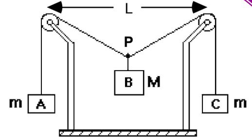
Start with just the string suspended between the pulleys (no central object), so that the string looks horizontal. Attach a central object and observe how the string sags. **Decide** on the origin from which you will measure the vertical position of the object.
