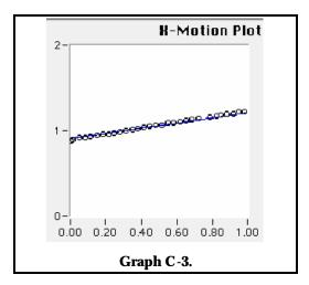
The line touching the data points in Graph G3 has a slope of 0.38 m/sec. This is the **minimum** possible slope for a line that fits the given data.
