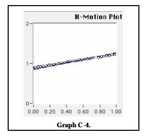
The line touching the data points in Graph C-4 shows a slope of 0.44 m/sec. This is the **maximum** possible slope for a line that fits the given data.You can estimate the uncertainty by calculating the average difference of these two slopes from that of the best-fit line. Therefore the uncertainty determined by graphs C-3 and C-4 is  $\pm$  0.03 m/sec.
