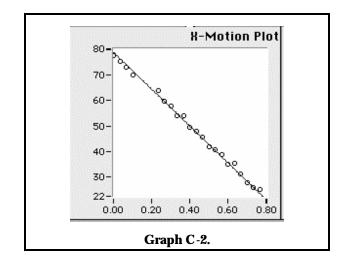
Finding the slope of any given curve with LabVIEW<sup>M</sup> should be easy after you have chosen the mathematical equation of the best-fit curve. Graphs C-3 and C-4 each show one possible line to describe the same data. From looking at these graphs, the estimate of the data's uncertainty is less than the diameter of the circles representing that data.
