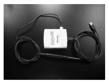
The tip of the measurement probe is embedded with a Hall Effect transducer chip (shown below as the white dot on the end of the probe). The chip produces a voltage that is linear with the magnetic field. The maximum output of the chip occurs when the plane of the white dot on the sensor is perpendicular to the direction of the magnetic field, as shown below:
