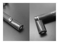
The measurement probes have swiveling tips to allow for more convenient data collection. Note: these tips are only meant to swivel in one direction. They will break of they are bent in the wrong direction, and they are very fragile, so it does not take much to do this. Please be very careful as these are costly to replace.
