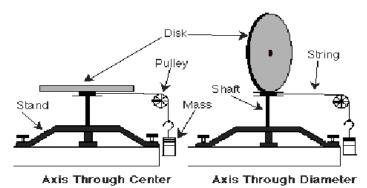
Below the disk there is a metal spool on the shaft to wind string around. A weight is hung from the other end of the string so that the weight can fall past the edge of the table. As the hanging weight falls, the string pulls on the spool, causing the disk/shaft/spool system to rotate. You will also have a meter stick, a stopwatch, a mass hanger, a mass set, a pulley clamp and the video analysis equipment in this experiment.
