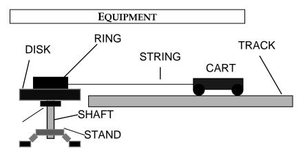
You will have a disk mounted horizontally on a sturdy stand, with a ring coaxially fastened on the disk. Together, the disk and the ring represent the flywheel. The disk and the ring rotate freely about a vertical shaft through their center.
