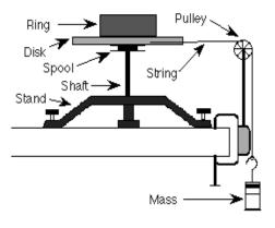
As the hanging weight falls, the string pulls on the spool, causing the ring/disk/shaft/spool system to rotate. You will also have a meter stick, a stopwatch, a pulley clamp, a mass hanger, a mass set and the video analysis equipment in this experiment.
