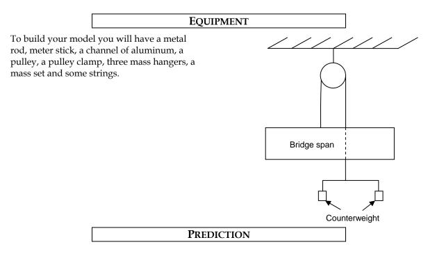
Predict the relationship between the weight of the bridge span and the total weight of the counterweights along with the metal rod. In addition, with the position of one of the counterweights fixed, find how the mass ratio of the counterweights varies with the position of the second counterweight in order for the entire setup to remain in static equilibrium. Assume that the bridge span is attached at the center of mass (CM) of the metal rod.
