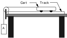
You can vary the mass of A and the Cart which are connected by a light string. Object A falls from a height shorter than the track's length. You will have a meter stick, a stopwatch, mass set, cart masses, a pulley & clamp, string and the video analysis equipment.
