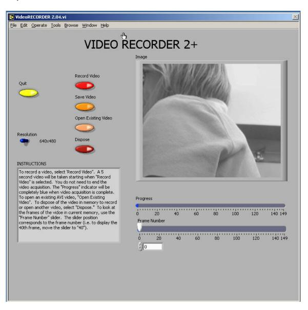
Using video to analyze motion is a two-step process. The first step is recording a video. This process uses the video software to record the images from the camera and compress the file. The second step is to analyze the video to get a kinematic description of the recorded motion.
