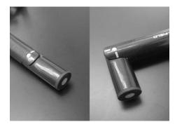
The measurement probes have swiveling tips to allow for more convenient data collection. Note: these tips are only meant to swivel in one direction. They will break of they are bent in the wrong direction, and they are very fragile, so it does not take much to do this. Please be very careful as these are costly to replace.
