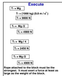
The force required to lift the block is the 3rd Law pair to  $T_{3}$ . It is 2450 N.
