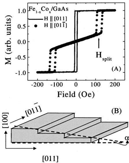
FIG. 1. (A) Typical hysteresis loops for  $Fe_{1-x}Co_x$  ( $x \sim 0.50$ ) on GaAs(100) for applied fields  $H$  parallel to  $[011]$  (solid curve) and  $[01\bar{1}]$  (points). The split field  $H_s$  is indicated by the arrow. (B) Schematic of a vicinal GaAs(100) substrate miscut toward  $(111)A$ . For  $(111)B$  miscuts, the steps are rotated  $90^\circ$ .
