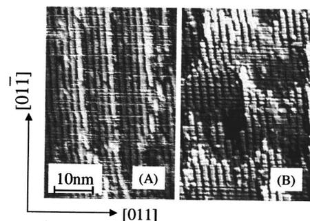
FIG. 4. Scanning tunneling microscope images of the surface steps on GaAs(100) miscut  $2^\circ$  toward  $(111)A$  (left) and  $(111)B$  (right).
